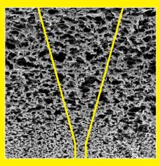
Hydrophilic PES membranes have a high internal porosity. They perform well at high flux with an excellent throughput of aqueous solutions over the entire pH range of 1-14. Their low level of extractables makes them suitable for environmental analysis. Thanks to their low non-specific protein binding, the PES membranes are recommended for filtering biological and pharmaceutical solutions.
