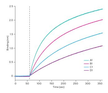
Figure 2: Four concentrations (10, 5, 2.5 and 1.25  $\mu$ g/mL) were chosen for evaluation while targeting 1 nm response over 300 seconds. The 1.25  $\mu$ g/mL concentration was chosen for further development. The baseline (first 60 seconds) and the loading step (60 to 360 seconds) for all four concentrations are shown.
