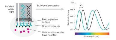
Figure 1: Relative intensity of the light reflection pattern from the two surfaces on the biosensor. Octet $^{\circ}$  BLI systems measure the difference in reflected light's wavelength ( $\Delta\lambda$ ) between the two surfaces.
