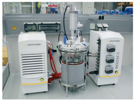
Figure 1: BIOSTAT<sup>®</sup> A setup for the *Escherichia coli* high cell density fermentation experiment
