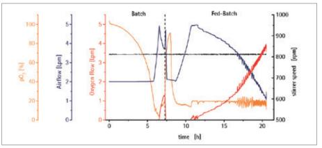
Figure 5: Oxygen partial pressure characteristics and control parameters. The  $pO_2$ , stirrer speed, gas flow rate and oxygen gas flow rate are shown.
